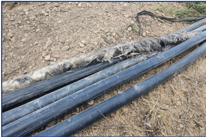
Figure 2 – The FlexSteel pipes that remained intact and the line that breached and burned during the initial attack response to the fire. This burned and ruptured pipe was moved to be compared to the new FlexSteel pipes.
