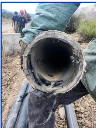
Figure 2 – The FlexSteel pipes that remained intact and the line that breached and burned during the initial attack response to the fire. This burned and ruptured pipe was moved to be compared to the new FlexSteel pipes.
